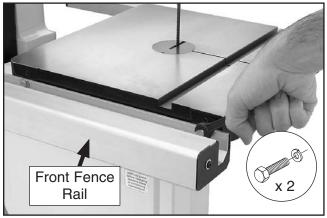
Figure 17. Installing front fence rail.
